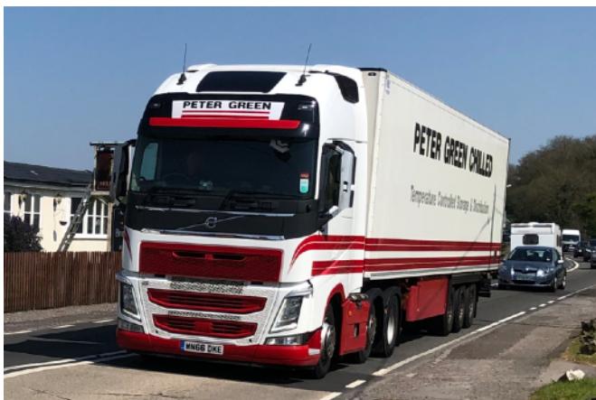
Figure 6: Peter Green Chilled HGV registered after 1 Sep 2016 - corner lights but no high level lights (LHS). Newer HGV registered after 1 Sep 2018 with high-level running lights in addition to high level corner lights.
